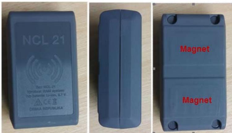
NCL21 unit is started automatically on the announced day and time at the beginning of the reconnaissance. It is set so that it works on the batteries for 24 hours if the unit moves and for 80 hours if it does not.
